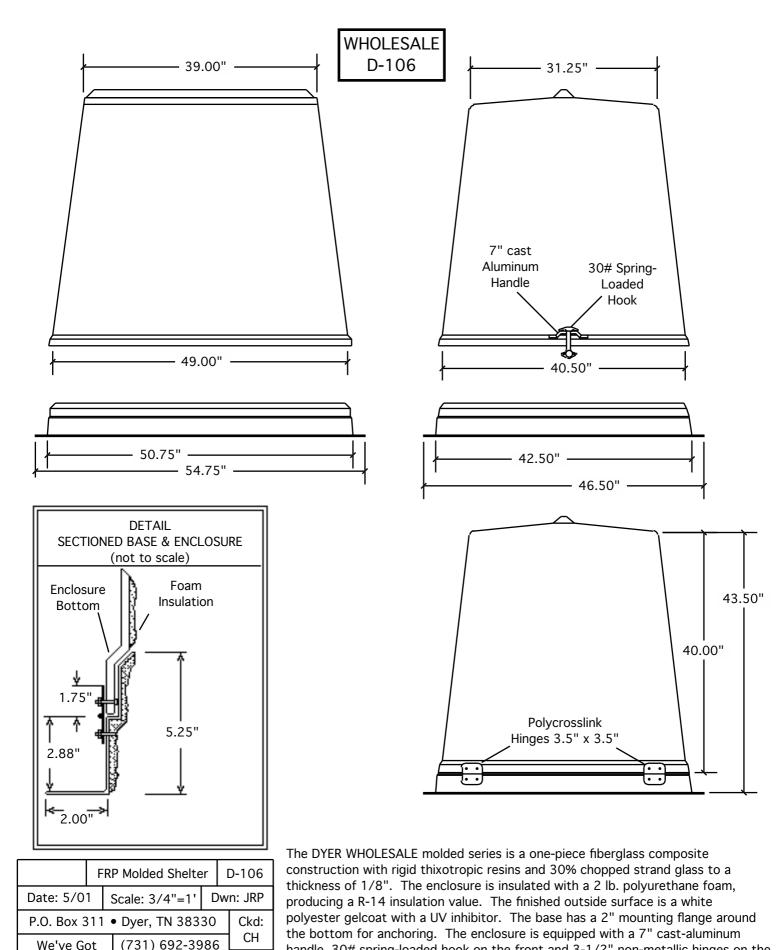
(731) 692-3986----<br/>handle, 30# spring-loaded hook on the front and 3-1/2" non-metallic hinges on the<br/>rear. Fasteners are 1/4" stainless steel nuts & bolts.<br/>Shipping weight: 45 lbs per cover plus pallet and cartoning.
